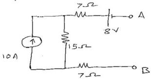
c. State maximum power transfer theorem. In the following network find the value of resistance  $R_L$  So that maximum power will transfer through it and also calculate this power.
