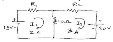
1. For the circuit shown below calculate current through  $10\Omega$  resistance using nodal analysis
