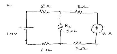
c. Find the voltages at nodes A and B in the network shown below
